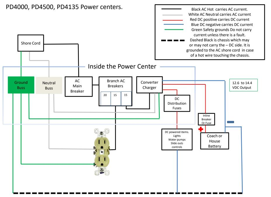
Chassis of RV or Trailer/Master System Ground
