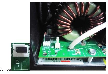
Lift it off the 2 pins and replace it over the center pin and the one on the LI side
