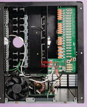
The Lithium switch is set to Lead Acid Batteries and it is located on the converter section next to the coil of the PD 4000 Series. The Lithium Switch on the PD 4500 Series is located on the DC Distribution Board. To switch converter into Lithium Mode (LI) simply slide the Lithium Switch up into the top position!
