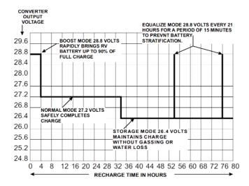
The integrated Charge Wizards ability to change the output voltage of the converter will significantly reduce the amount of time it takes to recharge your battery. The lower voltage for Storage Mode prevents gassing and reduces water loss during long-term storage.
