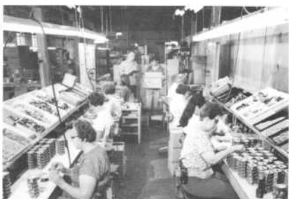
GAS REGULATOR ASSEMBLY LINE
