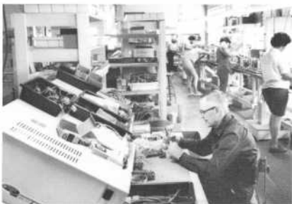
POWER CONVERTER ASSEMBLY LINE
