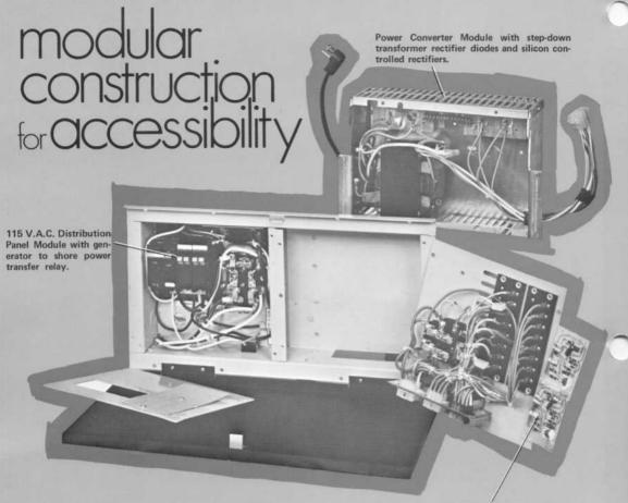
The Power Converter Module of the shore power system operates in the following manner: When your boat is connected to 115 V.A.C. the relay in the D.C. panel module automatically disconnects the batteries from the 12 volt electrical system and places them on charge. The Power Converter Module then supplies all the 12 volt power necessary to operate lights, fans, pumps, etc. This system ensures that your batteries will have a maximum charge when you leave the dock.
