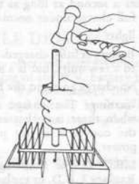
Removing Rectifier Diodes
